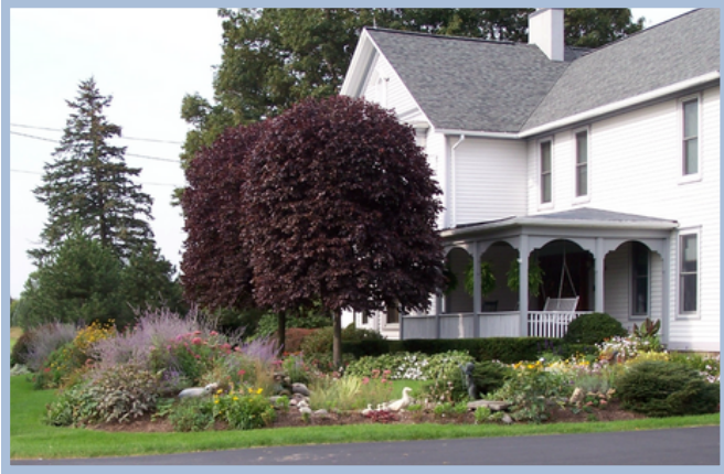
Rain garden intercepts roof runoff before driveway
